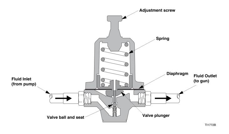
Fig. 2. Cutaway of Mechanical Fluid Pressure Regulator
